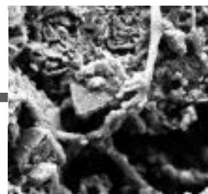
Detailed microphoto of the marble structure covered in black dust – Freedom Monument, Riga (LT).
